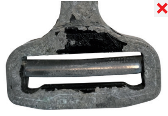
corrosion of the buckle after mortar splashing
