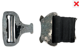
corrosion of the buckle after mortar splashing
