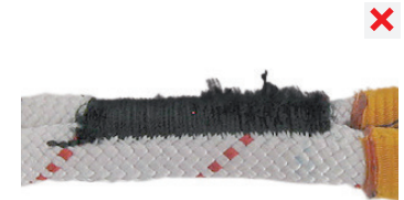
damaged strength seam
