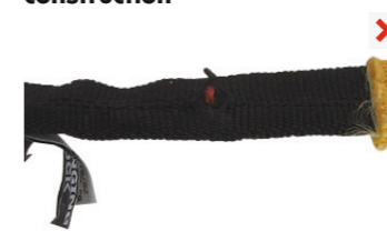
damaged webbing construction
