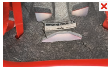
broken construction of the helmet absorber
