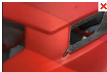
damaged helmet absorber
