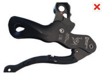
damaged regulation handle
