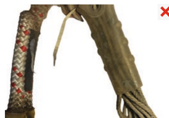
damaged sheath and core
