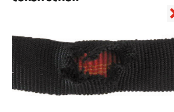
damaged webbing construction
