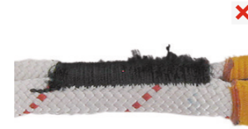
damaged strength seam
